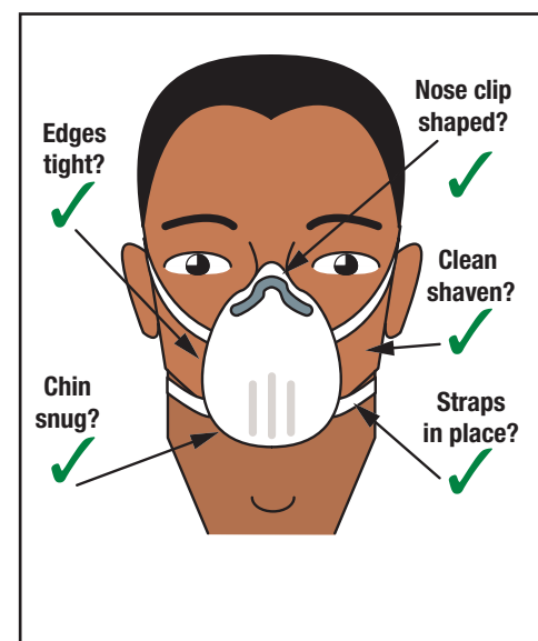
Check it! Check your mask before you put it on. Then do a fit check – for a proper fit each time
