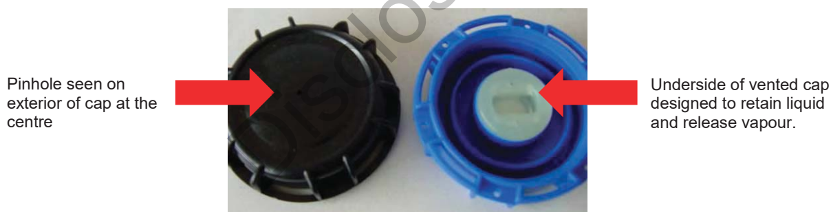
Figure 2 - example of cap with vent incorporated into its design.
