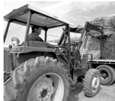
Figure 4. Tractor fitted with a FEL, specifically designed for loading/unloading hay bales.
