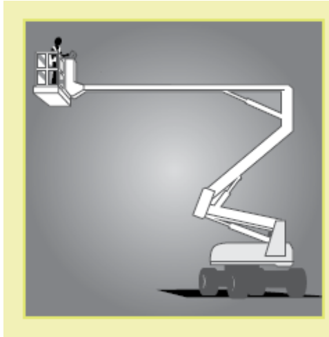
Figure 9: An example of a boom-type elevating work platform. The safety harness and lanyard assembly are not shown for purposes of clarity. The lanyard should be as short as possible and should be attached directly to the designated anchor point on the EWP, not to the handrail.
