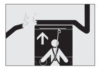
To travel past the cutout height, push the Override Switch while, at the same time, pushing either the Raise or Lower button.
