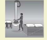
A vacuum operated lifting device can reduce the forces, awkward postures, and movements required to manually load products onto pallets.
