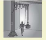
Using mechanical equipment, such as overhead cranes to lift and move very heavy objects eliminates the need to apply high force.
