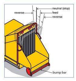
For extra protection, consideration should be given to retro-fitting existing wood chippers with an in-feed stop control device also known as a push bar or bump bar, along the bottom leading edge of the in-feed chute. This device should stop the in-feed rollers when a person uses body pressure to push against the bar.
