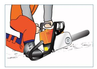
When starting a chainsaw with a hot engine, operators may choose the alternative method of:
