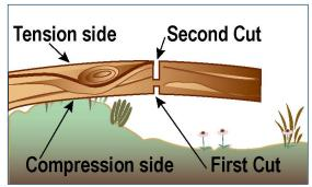
During the cutting process operators should continually assess the tensions and resultant movement to minimise the risk of jamming. Operators should be aware that a kickback hazard may occur if the upper tip of the guide bar is pinched in the cut. They should adjust their cutting techniques in response to any movement in the tree or limbs being cut.
