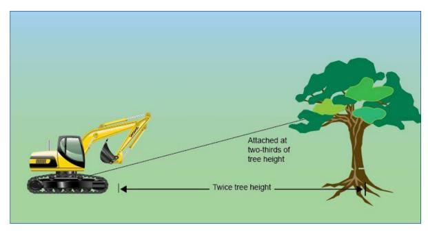
Powered mobile plant, for example excavators and bulldozers, can be used to push trees in a desired fall direction provided they:
