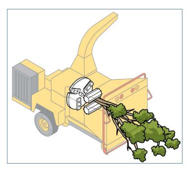
Workers operating wood chippers can also become entangled while standing beside or in front of the in-feed chute or while they are feeding material into the wood chipper. If ropes, clothing or gloves are caught on a branch being fed into the wood chipper, the worker can be dragged past the safety curtain and the in-feed rollers onto the cutting blades.
