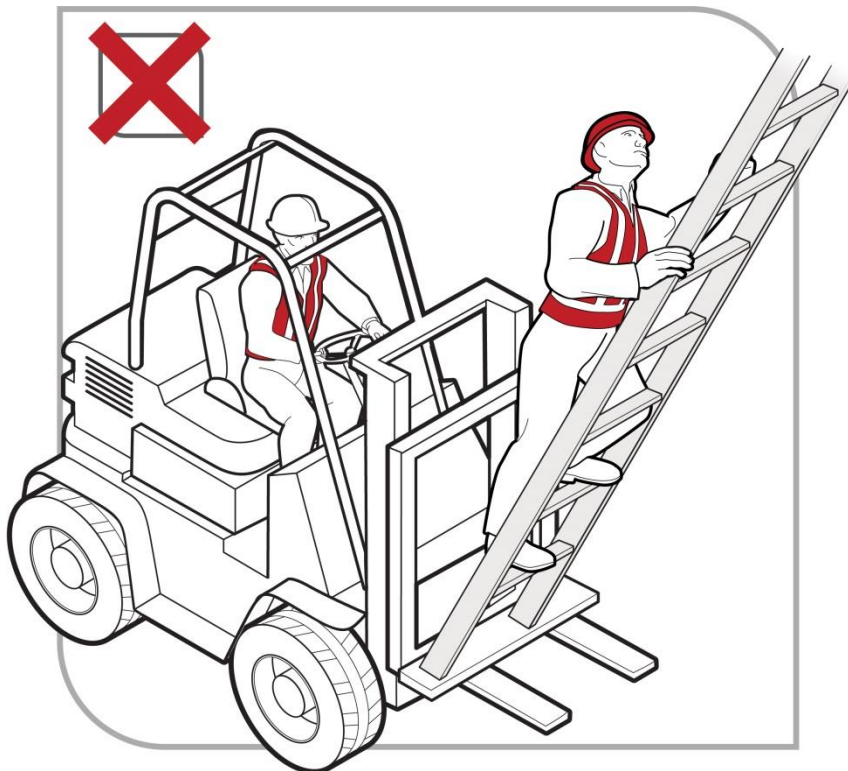
Figure 15 Unacceptable practice with ladder on forklift
