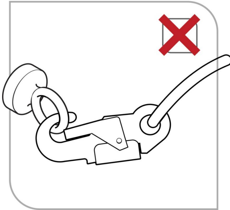
Figure 22 Roll-out on a small diameter eyebolt
